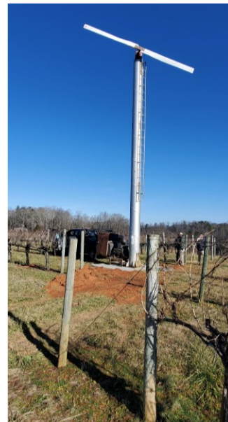
Figure 1: A stationary wind machine in North Carolina. (Photo: Eric Case)
